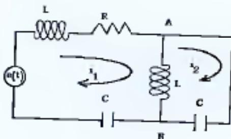
$$5^{\circ}) \text{ Cas où } \omega = \omega_0 = \frac{1}{\sqrt{LC}} \Rightarrow Z_{AB} = \infty \Rightarrow i_1 = 0 \Rightarrow \dot{X}_1 = 0. \text{ Ou bien} \quad (02pt)$$
