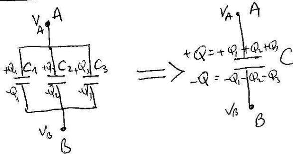
$$V_1 = V_A - V_B = \frac{Q_1}{C_1} \quad , \quad V_2 = V_A - V_B = \frac{Q_2}{C_2} \quad , \quad V_3 = V_A - V_B = \frac{Q_3}{C_3}$$
